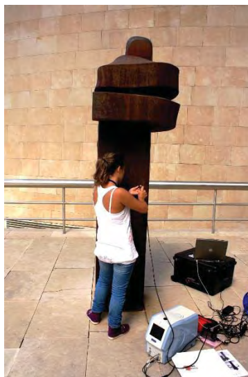
Figure 1. Portable Raman spectroscopy in an in-situ steel sculpture study.
