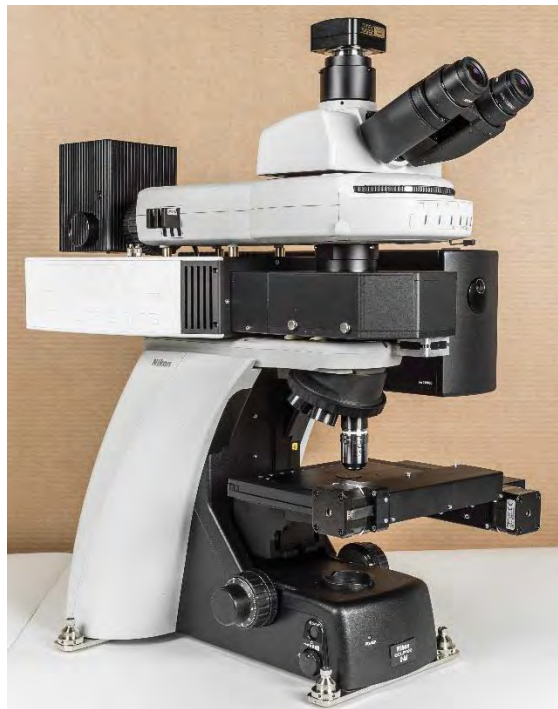
Figure 1: Confocal Raman microscope Confotec ® MR200 (SOL instruments)
