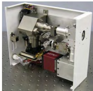
Figure 1: Inside the Compact Integrated Raman Spectrometer [2].
