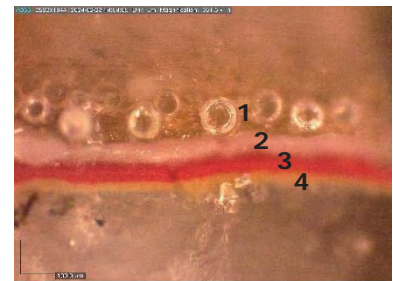
Figure 1. Cross-section of a retroreflective sheet sample taken from the sculpture in Fig. 1, comprising of four layers: 1) silica beads, 2) adhesive, 3) red color, 4) yellow color.
