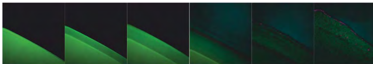
Figure 1: Dissolution of PVPVA (polymer, green) – ritonavir (drug, magenta) film at 20% drug loading. Dissolved product shown in cyan. Time points 1-2-5-10-15 minutes after adding the phosphate buffer solution (pH 6.8). First, the film wets and then forms a gel layer in which the drug separates. Image size 212x212 \mu\text{m} .
