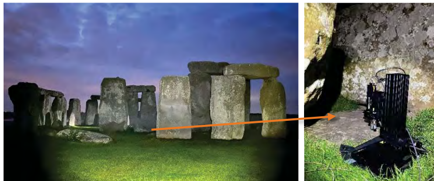
Figure 1. Using a Raman microscope on the Altar Stone at Stonehenge
