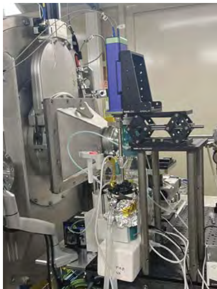
Figure 1: Photograph of LFR system coupled with synchrotron small angle X-ray scattering beamline at MAX IV illustrating the analytical flexibility of the technique.
