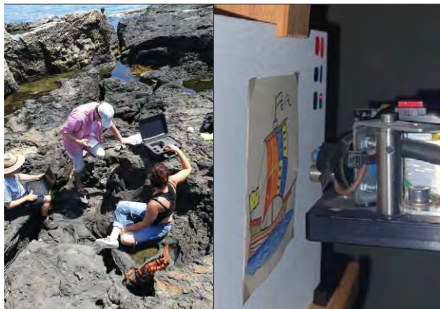
Figure 1: Implementation of mobile Raman instrumentation for in situ analysis (left) and using similar instruments for macro-Raman mapping of an artefact (right)
